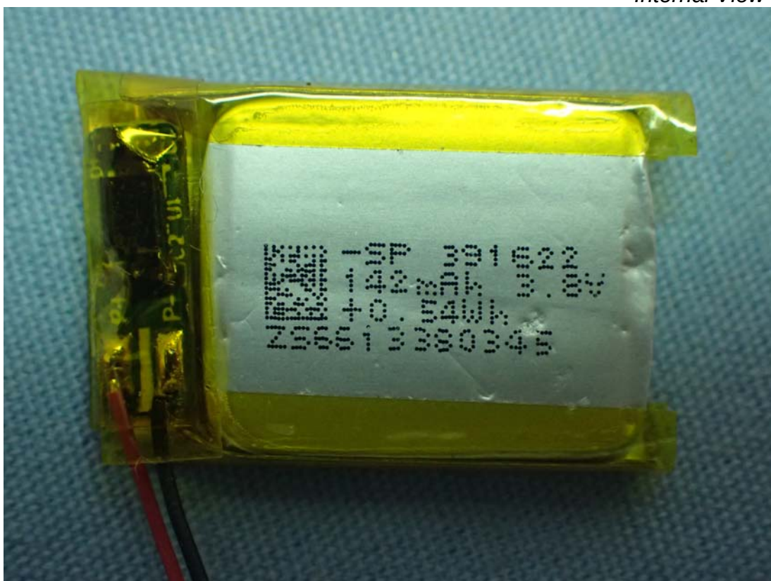
Figure 8 Internal View (Battery)
