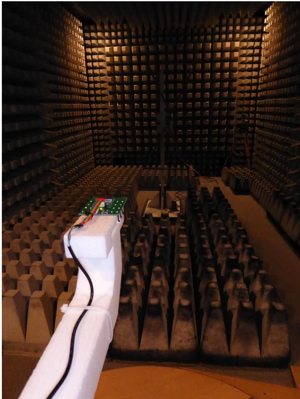
160903_03: Test setup - Radiated emission anechoic chamber
