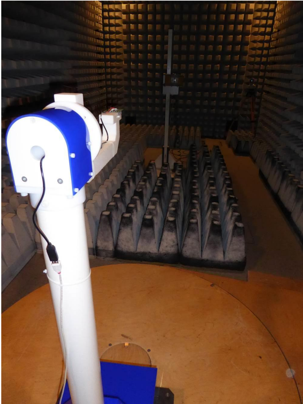
160903_04: Test setup - Radiated emission anechoic chamber
