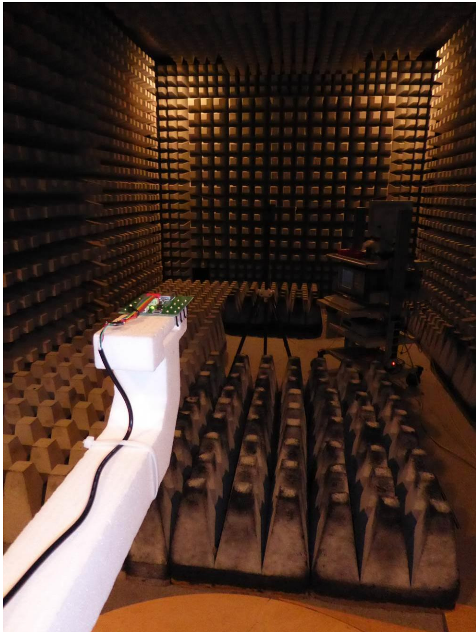
160903_05: Test setup - Radiated emission anechoic chamber
