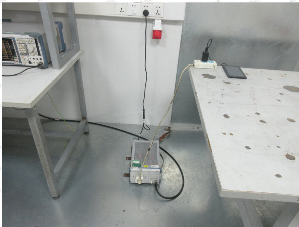
Photo of Conducted Emission Measurement
