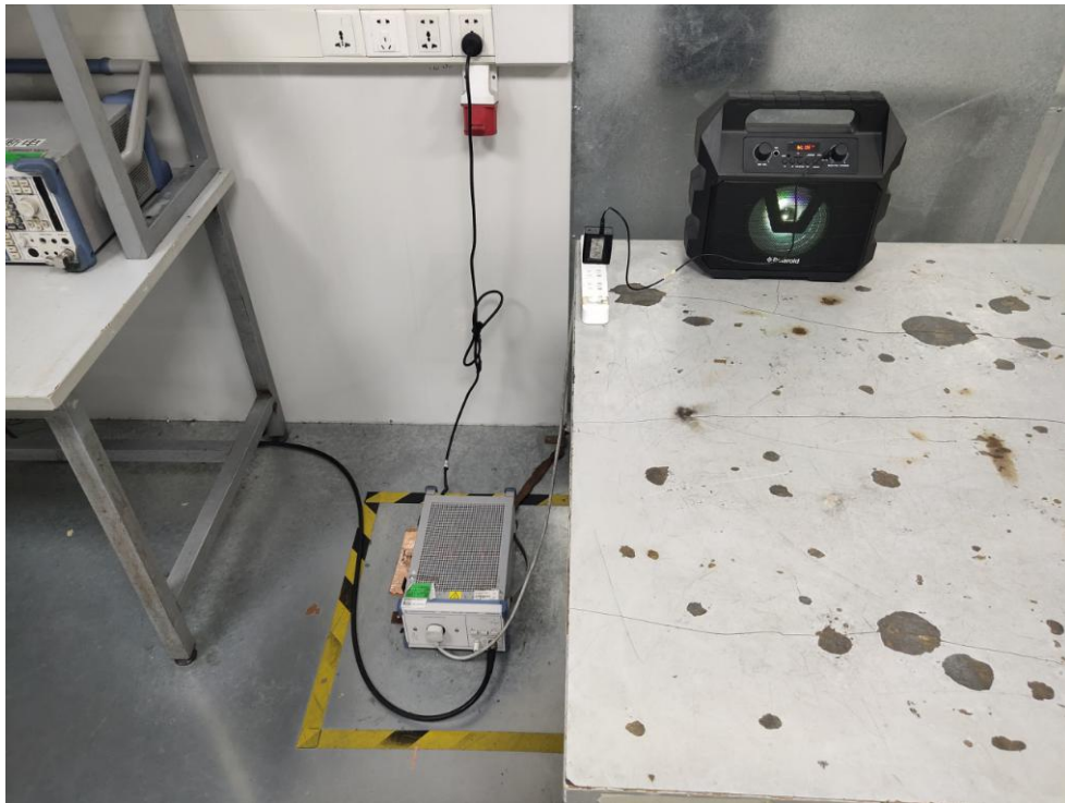
FCC ID: 2AIP7PBT9518 Photo of Power Line Conducted Emission Test
