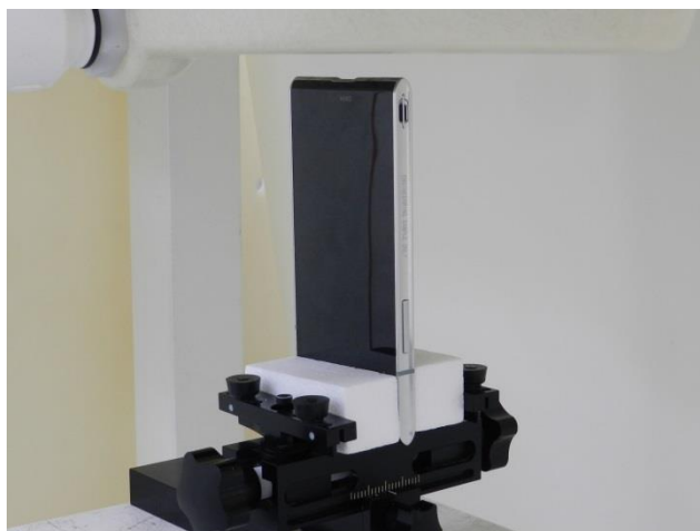
Bottom Side, Test Separation 10 mm
