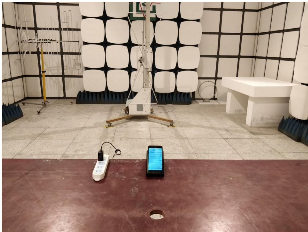
Radiated Emission below 1GHz-AC adapter charge mode
