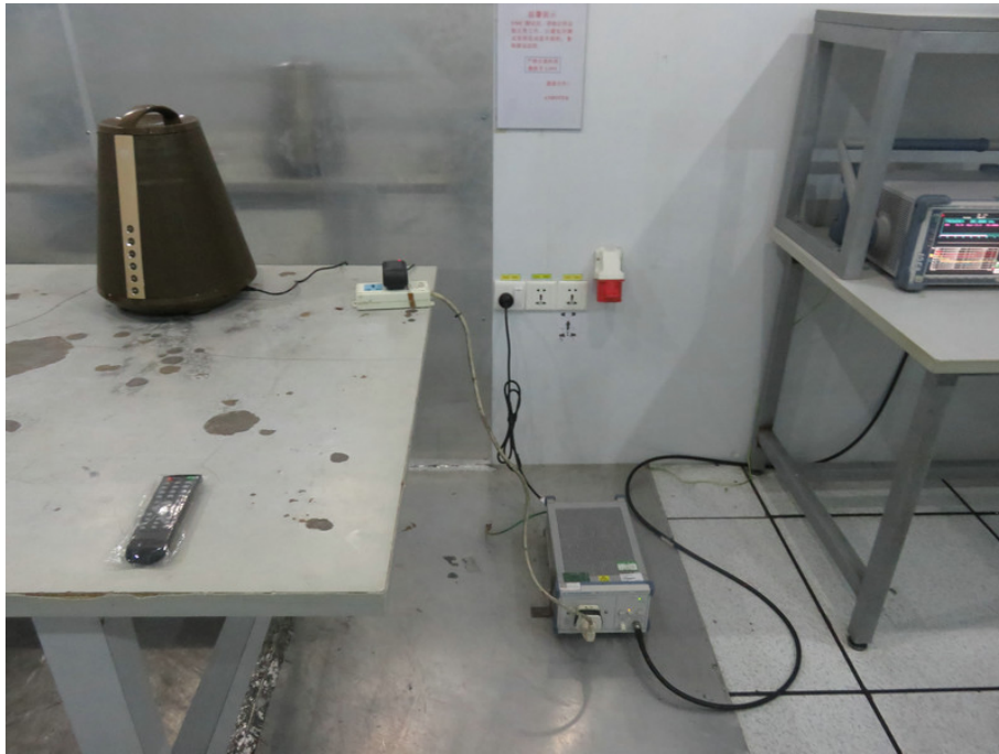
1 Photo of Power Line Conducted Emission Measurement
