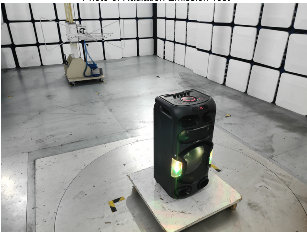
Photo of Radiation Emission Test
