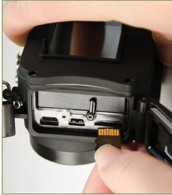
4. INSERT MICRO SD CARD (Up to 64GB class 10 microSD card)
