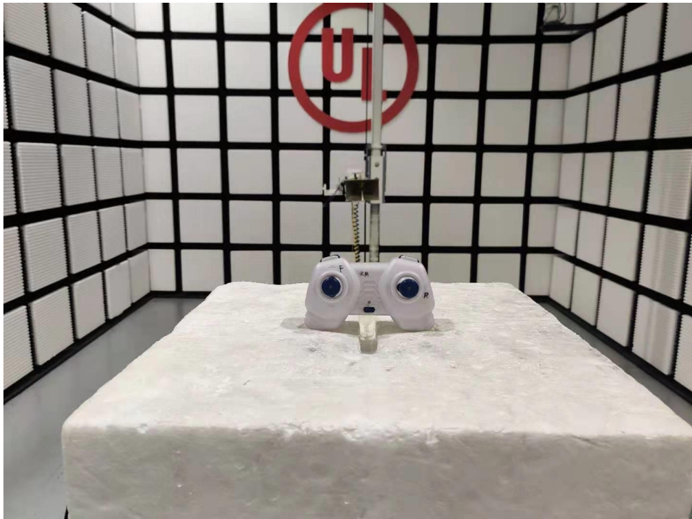
Radiated Disturbance Setup (Above 1 GHz – Y axis)
