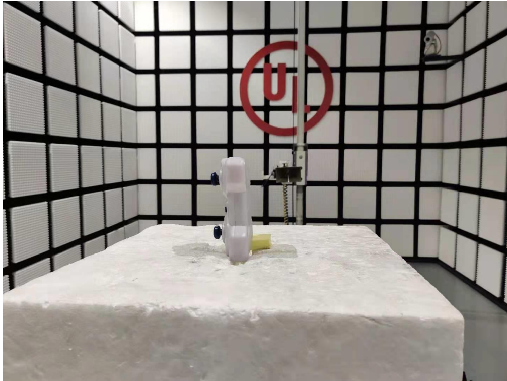
Radiated Disturbance Setup (Above 1 GHz – Z axis)
