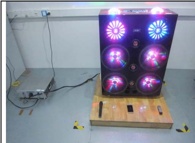
Conducted Emissions Test Setup Front View
