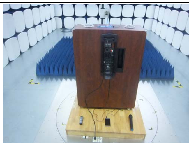
Radiated Emissions Test Setup Above 1GHz
