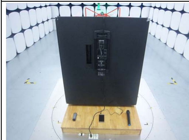
Radiated Emissions Test Setup Below 1GHz
