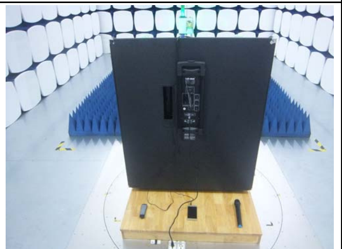
Radiated Emissions Test Setup Above 1GHz
