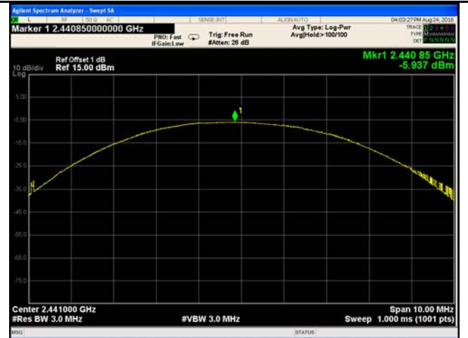
GFSK Output power - Mid CH 2441
