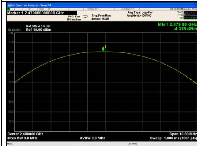
GFSK Output power - High CH 2480
