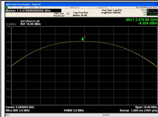
8DPSK Output power - High CH 2480
