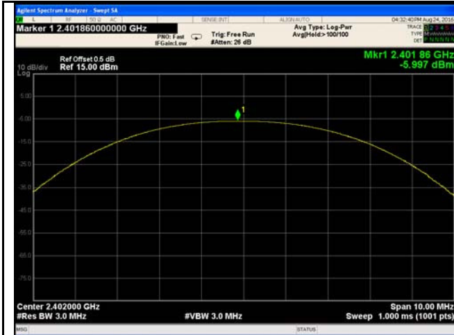
GFSK Output power - Low CH 2402
