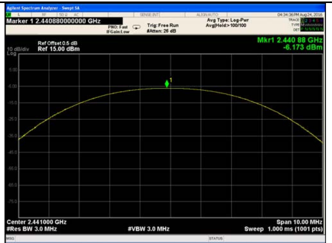
8DPSK Output power - Mid CH 2441
