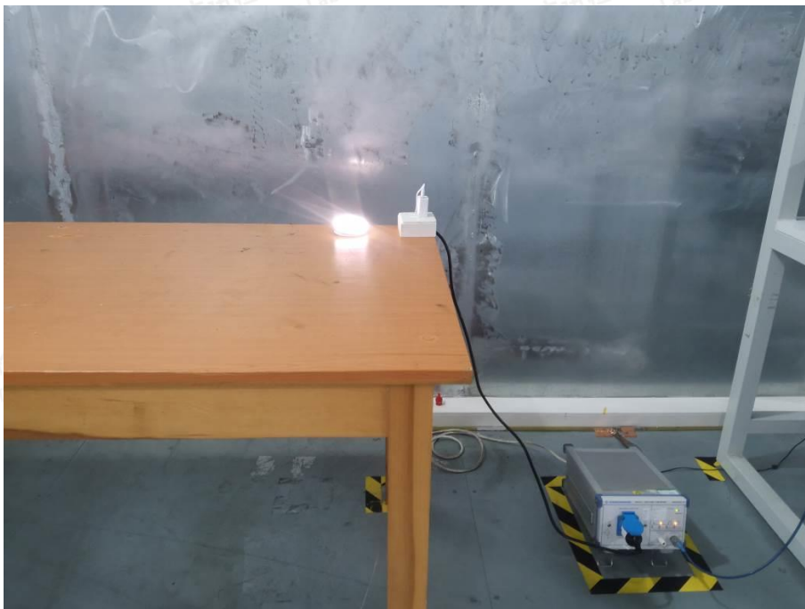
Photo of Power Line Conducted Measurement
