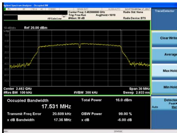
(802.11N20) 6dB Bandwidth plot on channel 11
