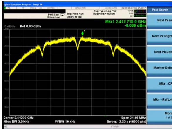
(802.11b) PSD plot on channel 6
