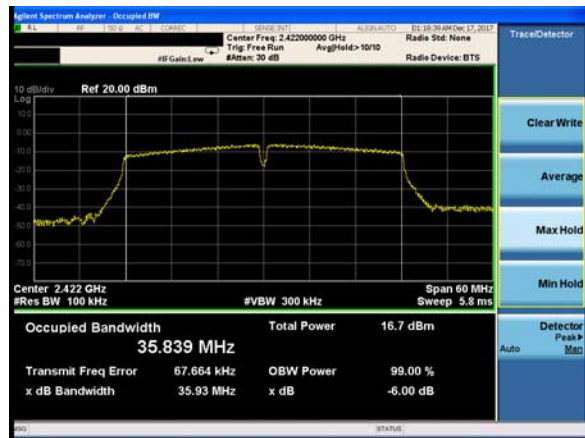
(802.1140) 6dB Bandwidth plot on channel 6
