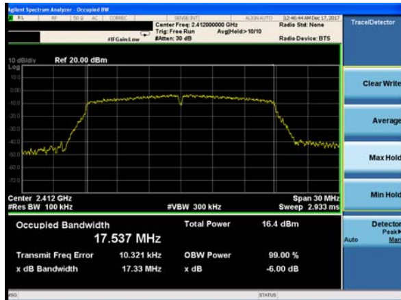
(802.11 N20) 6dB Bandwidth plot on channel 6
