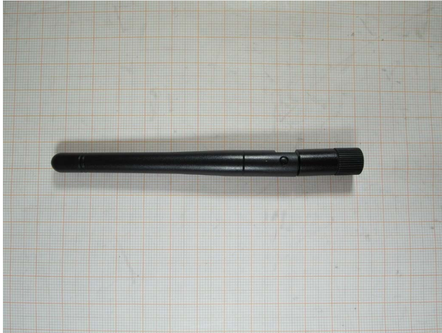
Photo 7: DelockRP-SMA_88395 - antenna 1 - omnidirectional dipole antenna
