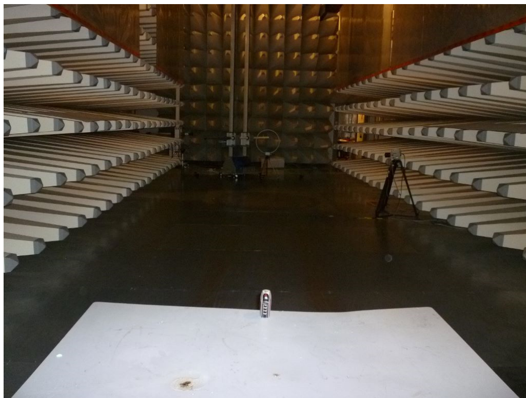
Set-up for Radiated Emission (Model: 3834)
