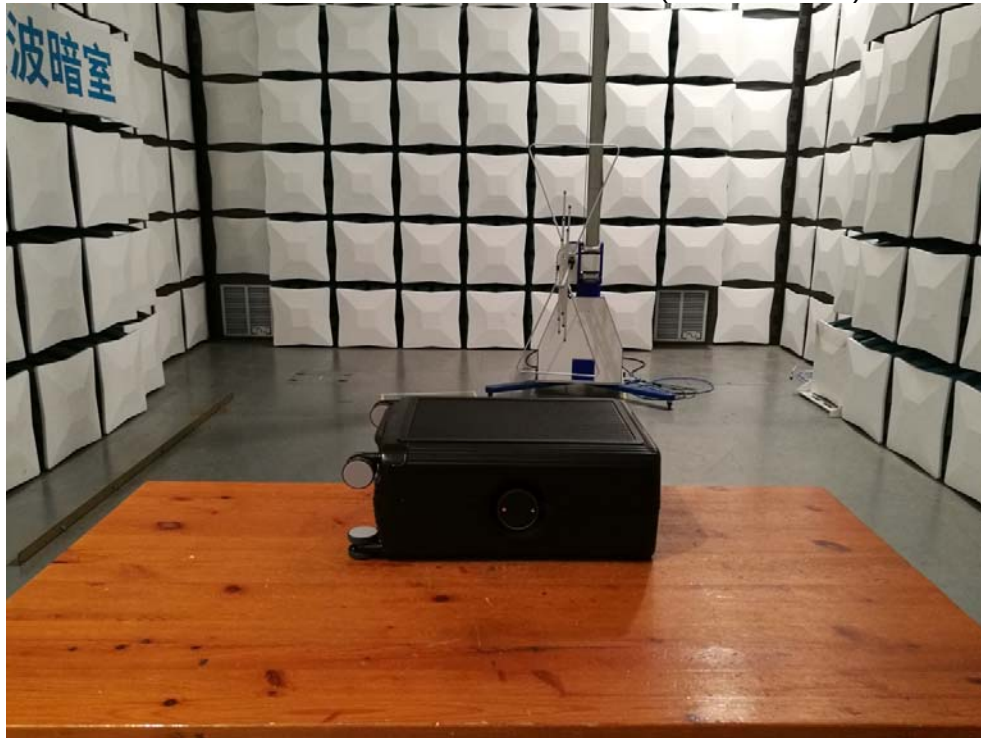
RADIATED RF MEASUREMENT SETUP (Above 1 GHz)
