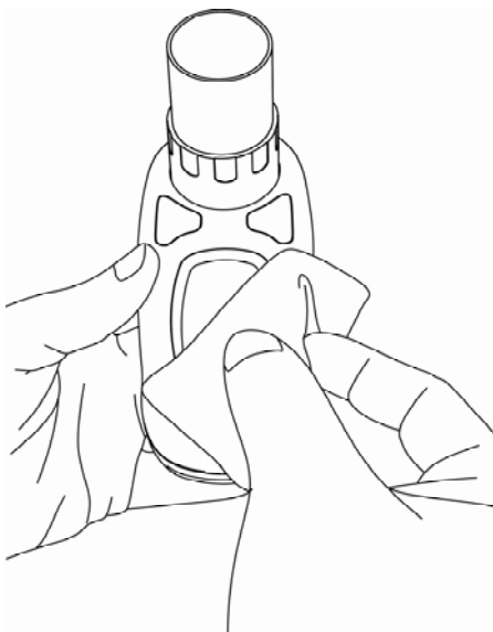
Figure3-4 cleaning to main unit
