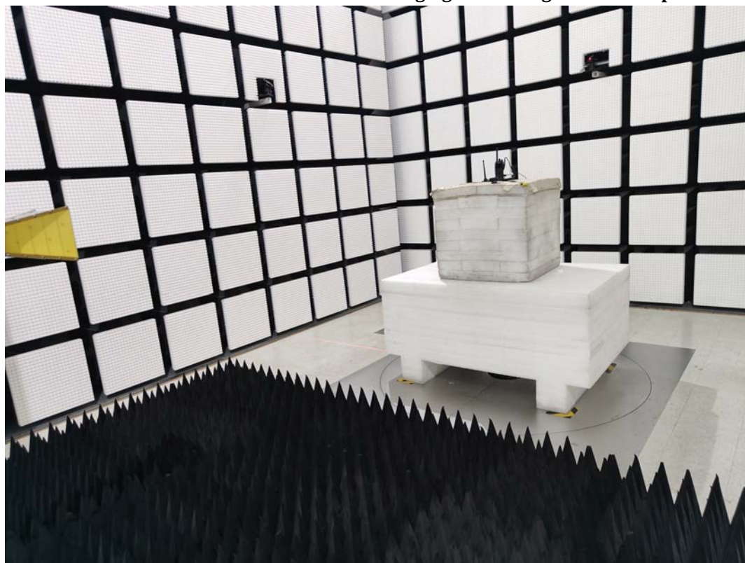
Radiated Emission Above 1GHz View Charging Dock + Big Hand Microphone
