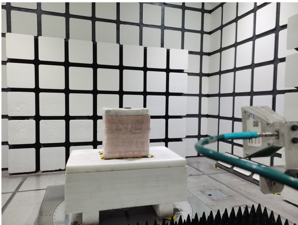
Radiated Emissions View (18-25 GHz)
