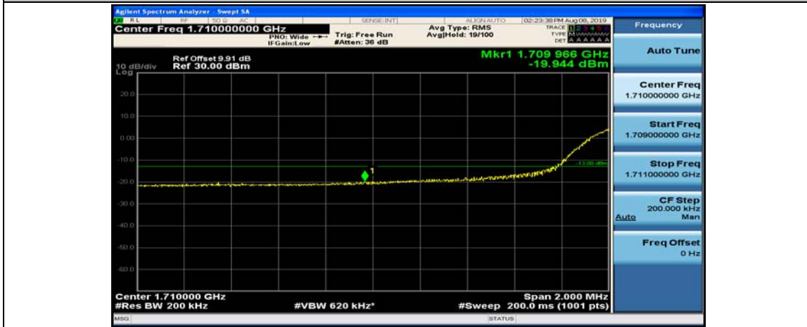
(Channel Bandwidth:20 MHz)_LCH_QPSK_50RB#25
