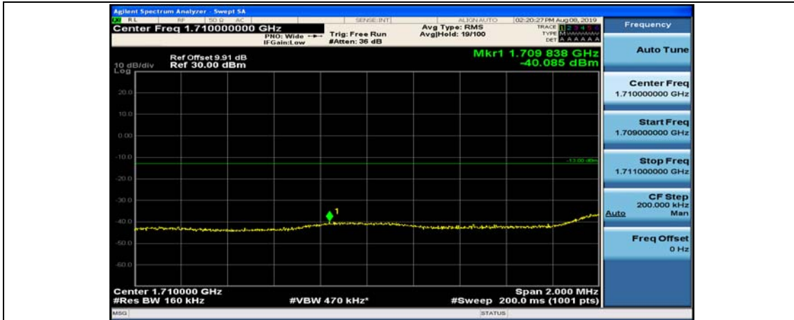
(Channel Bandwidth:15 MHz)_LCH_QPSK_75RB#0
