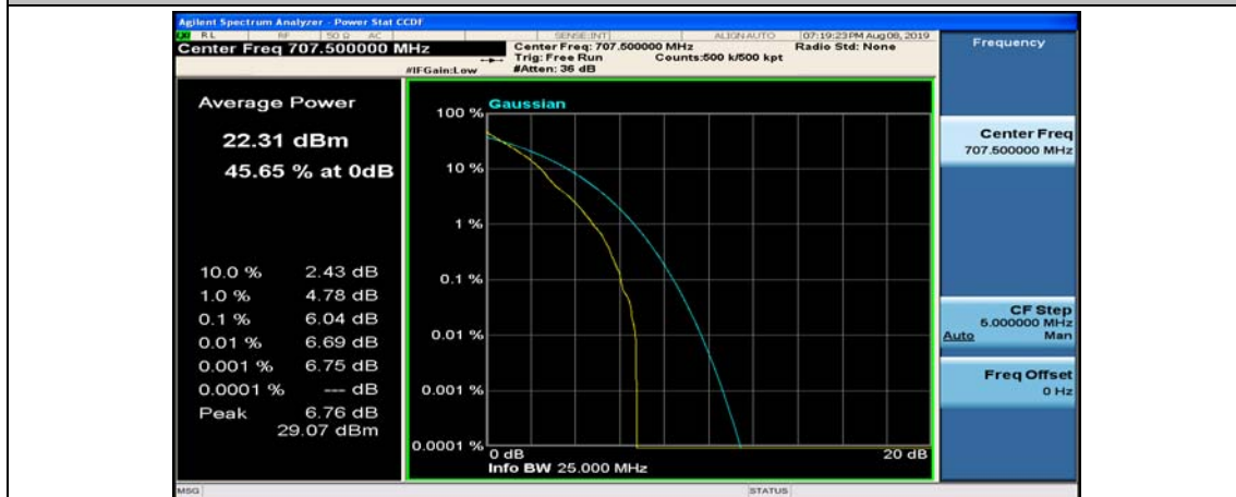
(Channel Bandwidth: 3 MHz)_MCH_QPSK_1RB#14
