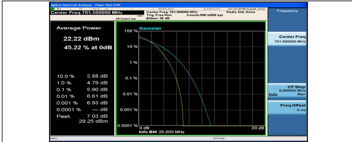
(Channel Bandwidth: 5 MHz)_MCH_16QAM_1RB#0
