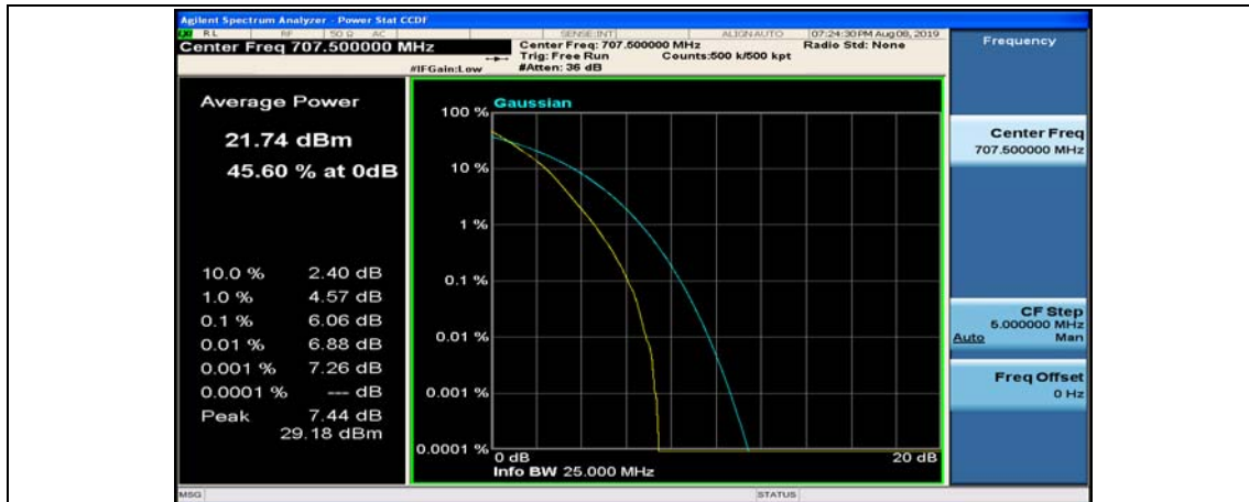
(Channel Bandwidth: 5 MHz)_MCH_QPSK_25RB#0
