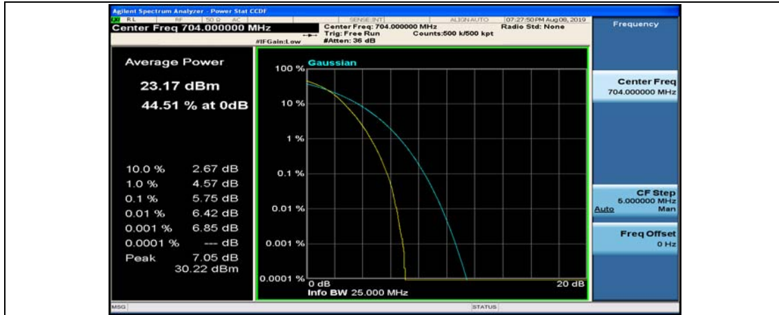
Channel Bandwidth: 10 MHz_MCH_QPSK_1RB#0
