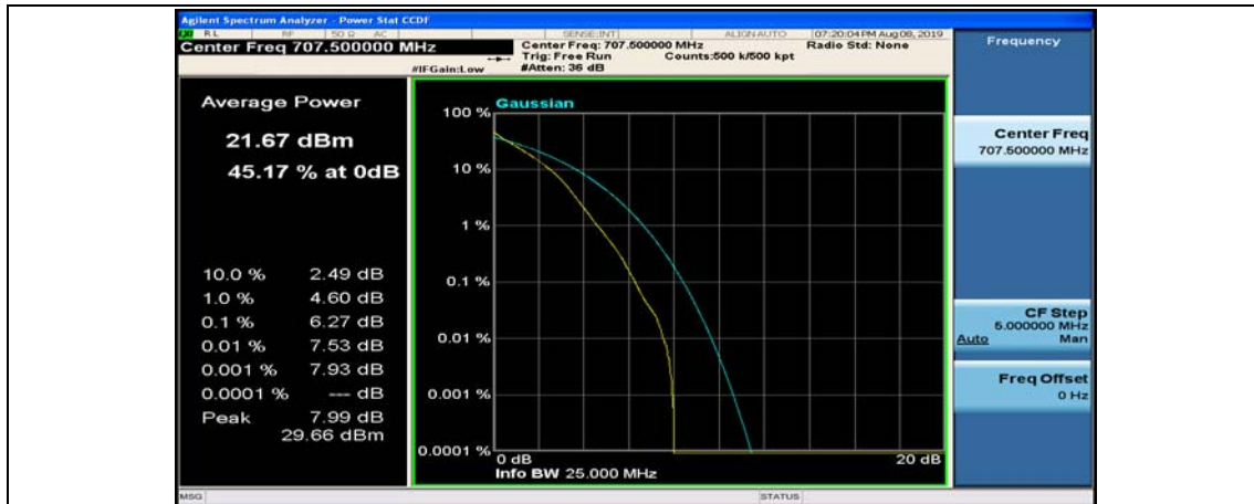
(Channel Bandwidth: 3 MHz)_MCH_QPSK_15RB#0
