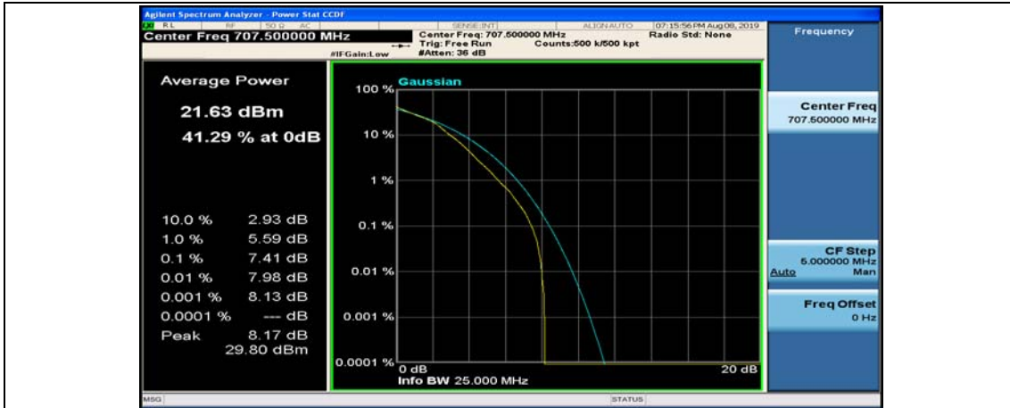
(Channel Bandwidth: 1.4 MHz)_MCH_16QAM_6RB#0
