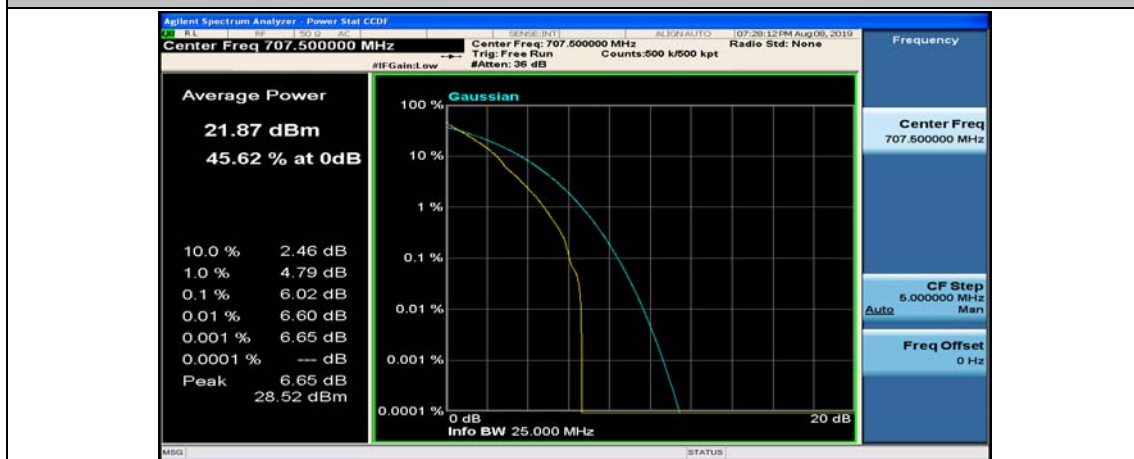
Channel Bandwidth: 10 MHz_MCH_QPSK_1RB#49
