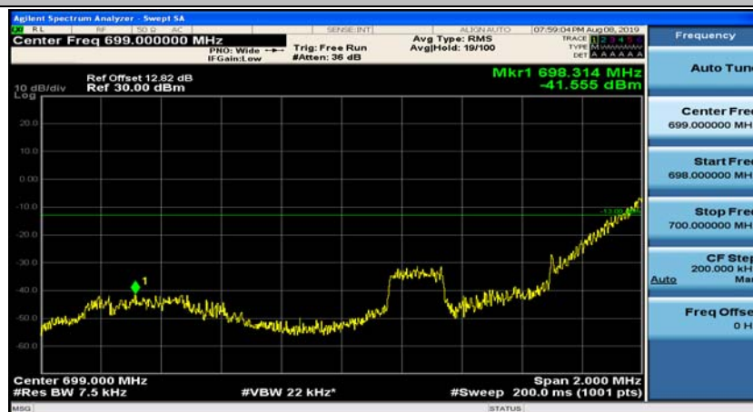
(Channel Bandwidth: 1.4 MHz)_LCH_QPSK_1RB#5
