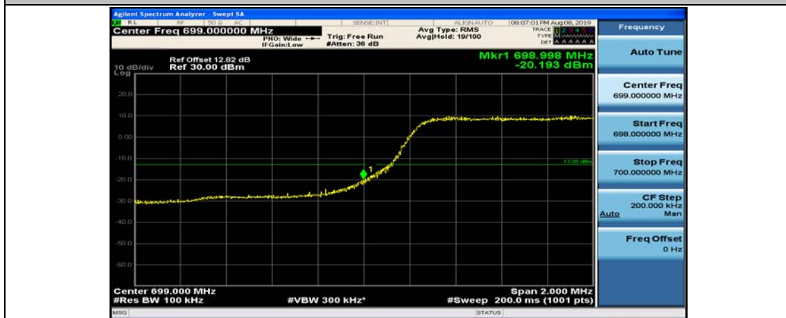
(Channel Bandwidth: 5 MHz)_LCH_QPSK_25RB#0
