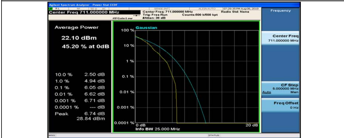
Channel Bandwidth: 10 MHz_HCH_QPSK_1RB#24
