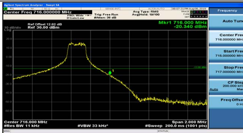
(Channel Bandwidth: 5 MHz)_HCH_QPSK_12RB#0
