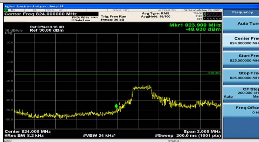
(Channel Bandwidth: 3 MHz)_LCH_16QAM_8RB#0
