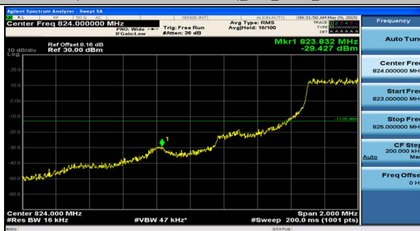
(Channel Bandwidth: 1.4 MHz)_LCH_QPSK_6RB#0
