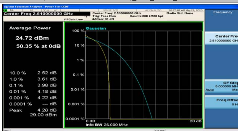
(Channel Bandwidth:20 MHz)_LCH_QPSK_50RB#0
