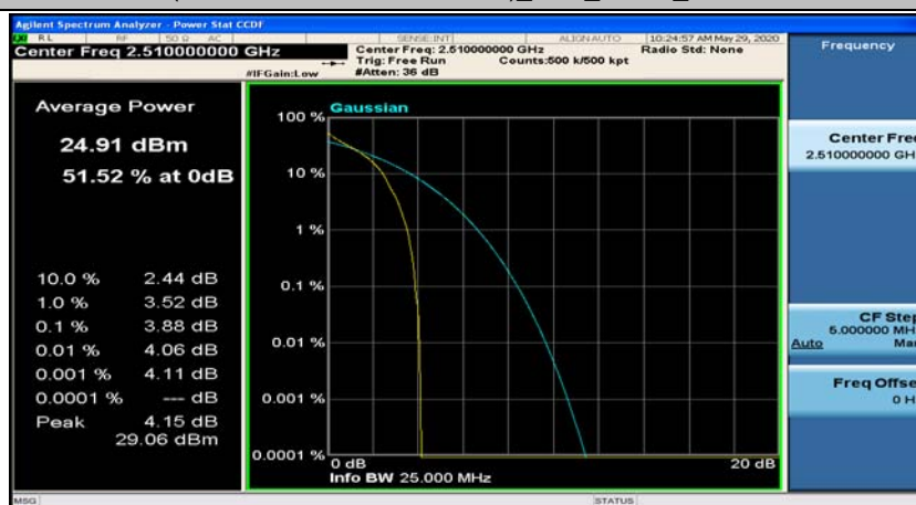
(Channel Bandwidth:20 MHz)_LCH_QPSK_1RB#49
