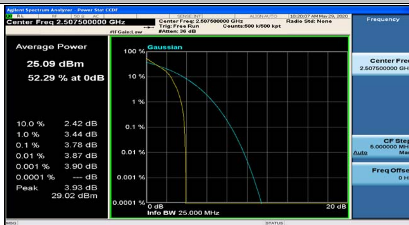
(Channel Bandwidth:15 MHz)_LCH_QPSK_1RB#37
