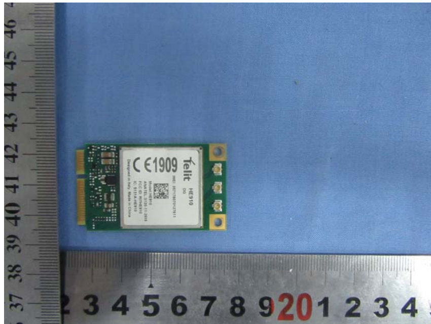
EUT – 2G/3G Module Top View
