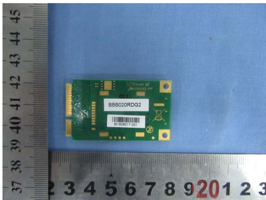
EUT – 2G/3G Module Bottom View
