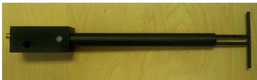
Figure 1 – MVG COMOSAR Validation Dipole
