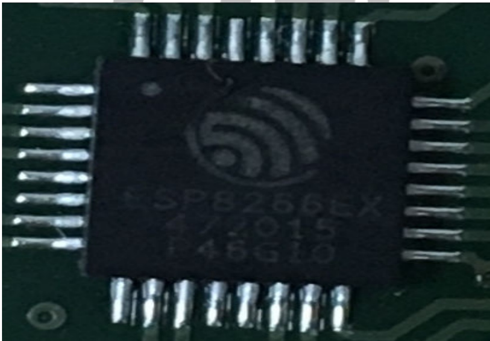
EUT –Wi-fi chip View
