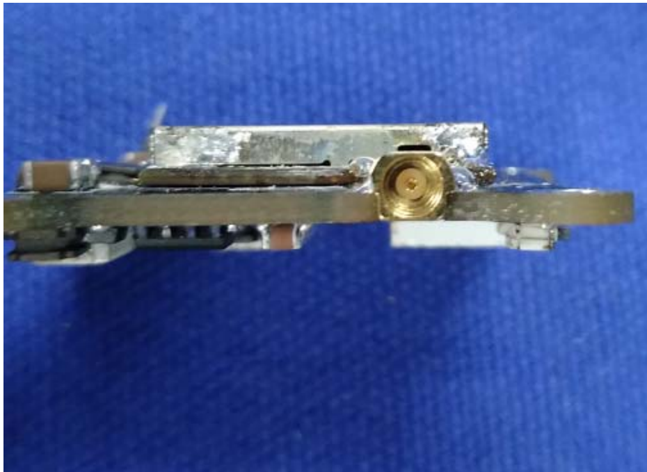
EUT – Equipment Antenna Connector (SMA Female) View
