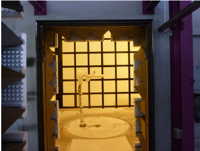
Photo 1: EUT at the anechoic chamber
