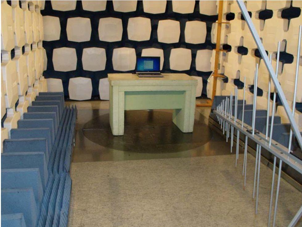
Figure 3: Radiated emission test from 30 MHz to 1 GHz
