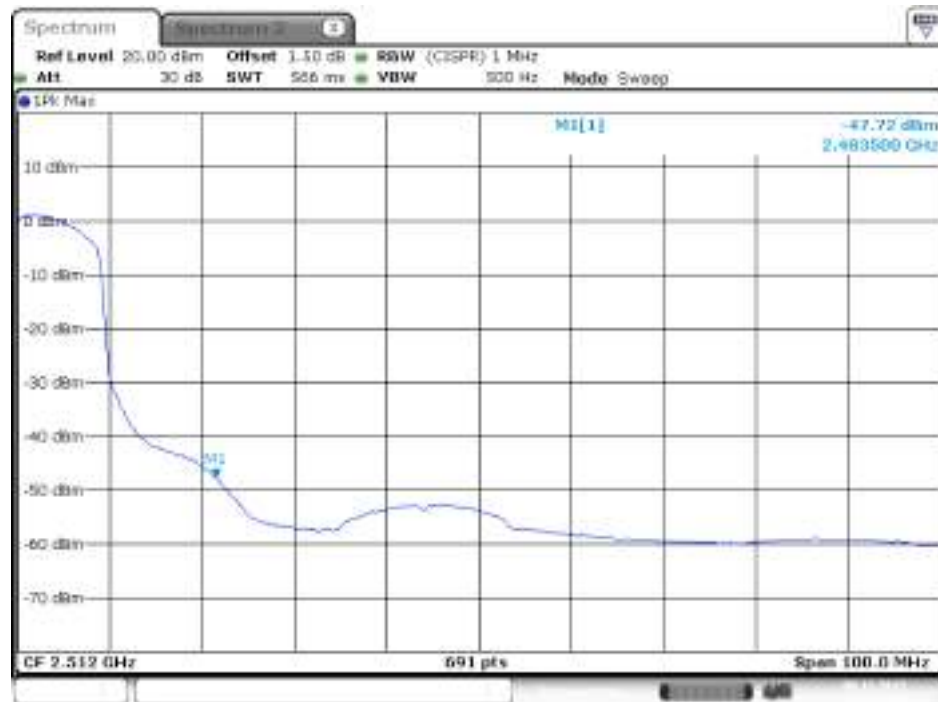
Plot on Configuration IEEE 802.11n MCS0 HT20 / 2462 MHz / Average / Chain 1
