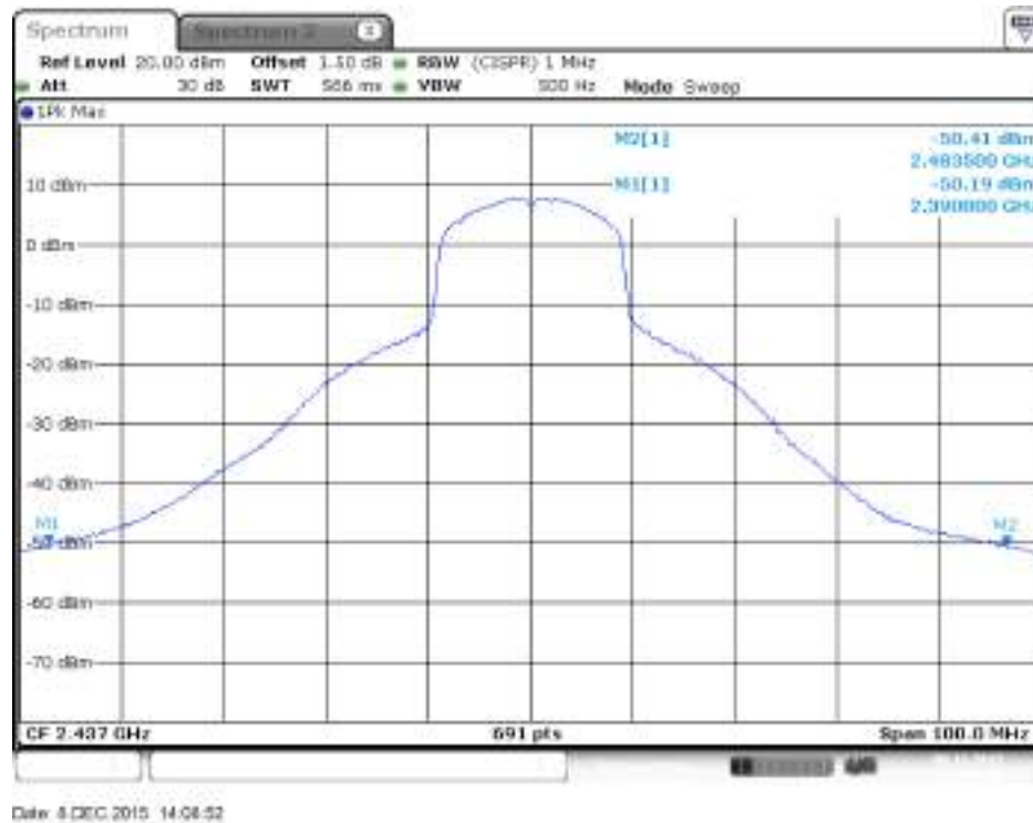
Plot on Configuration IEEE 802.11n MCS0 HT20 / 2437 MHz / Peak / Chain 1
