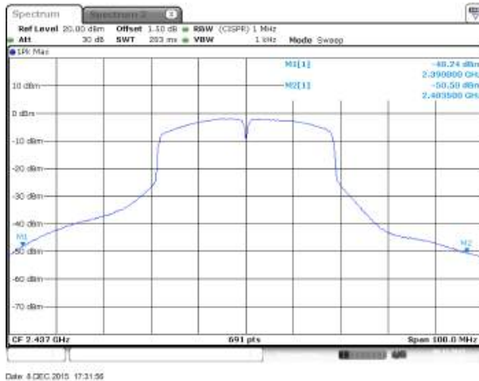
Plot on Configuration IEEE 802.11n MCS0 HT40 / 2437 MHz / Peak / Chain 2
