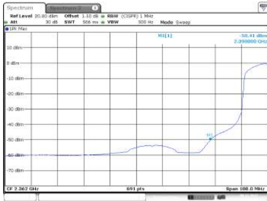
Plot on Configuration IEEE 802.11n MCS0 HT20 / 2412 MHz / Average / Chain 1
