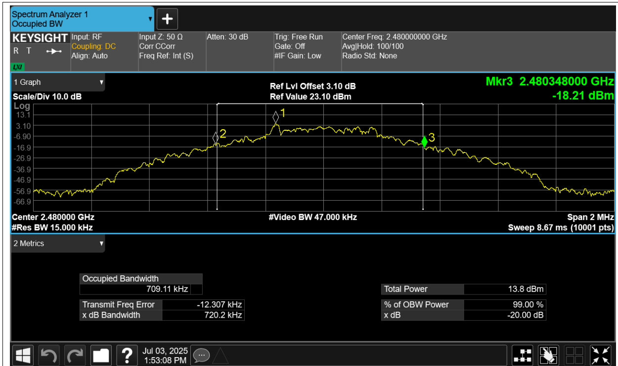
-20dB Bandwidth NVNT 2-DH1 2402MHz Ant1
