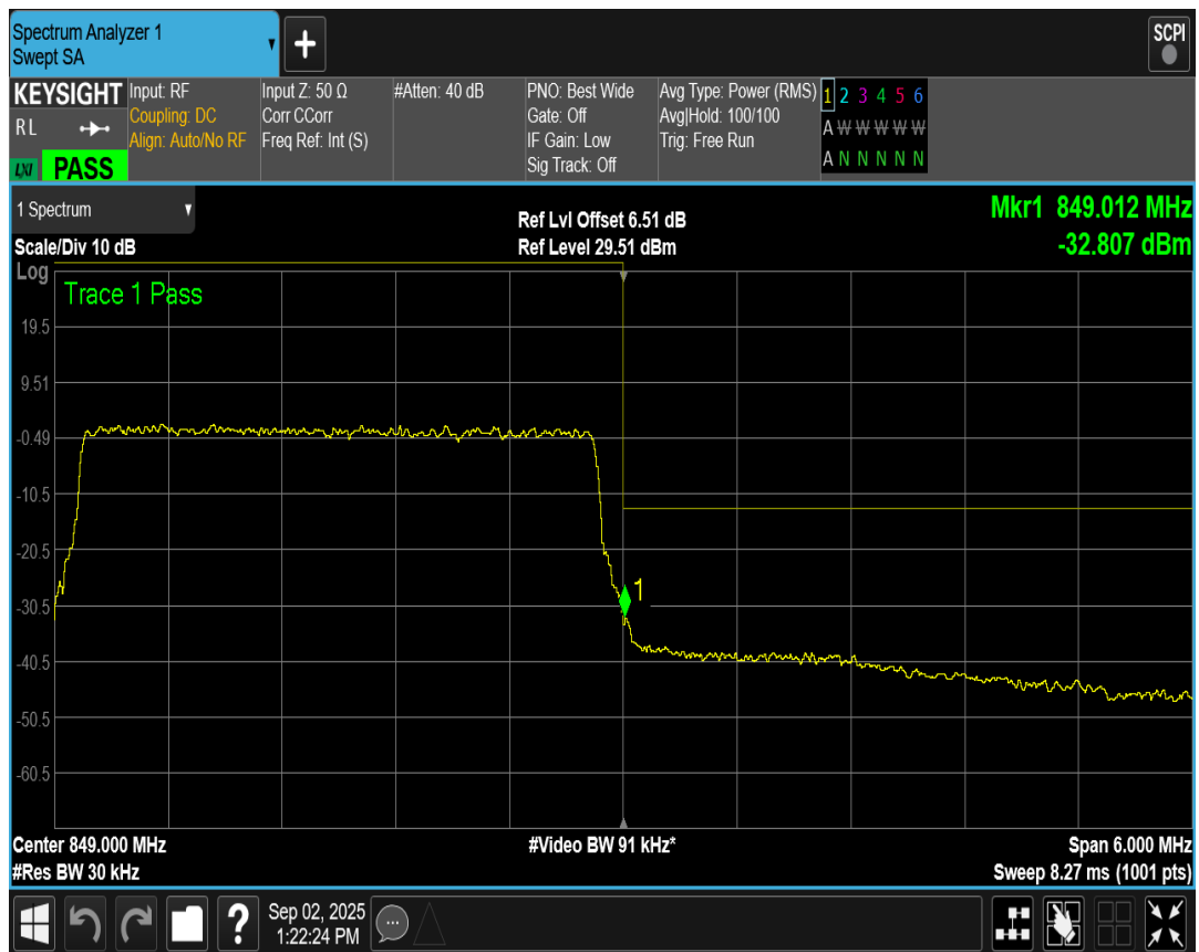
Band5 QPSK BW=3MHz Channel=20415 RB Size=15 Position=#0
