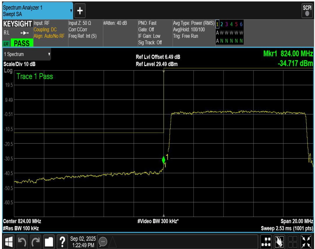
Band5 QAM16 BW=10MHz Channel=20600 RB Size=50 Position=#0
