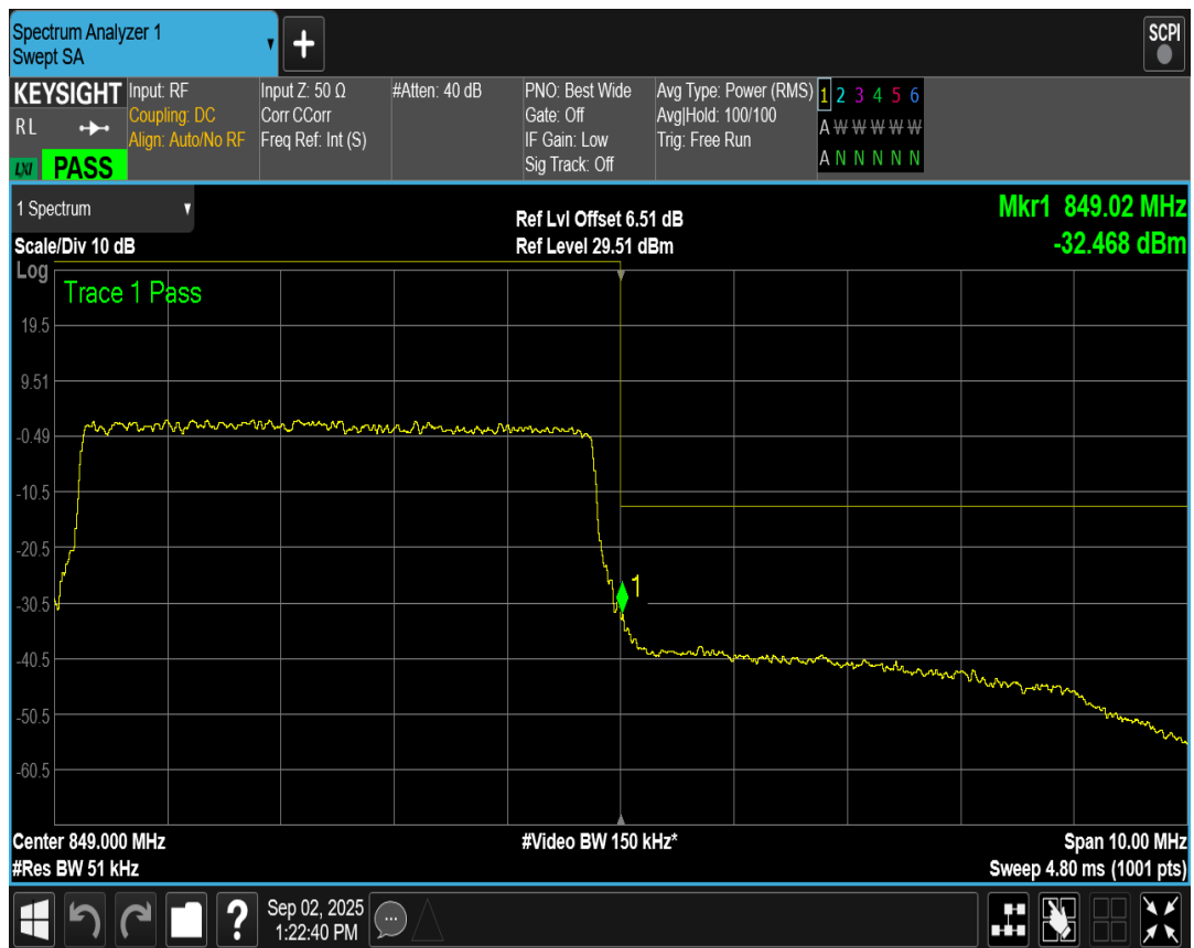
Band5 QPSK BW=1.4MHz Channel=20407 RB Size=6 Position=#0
