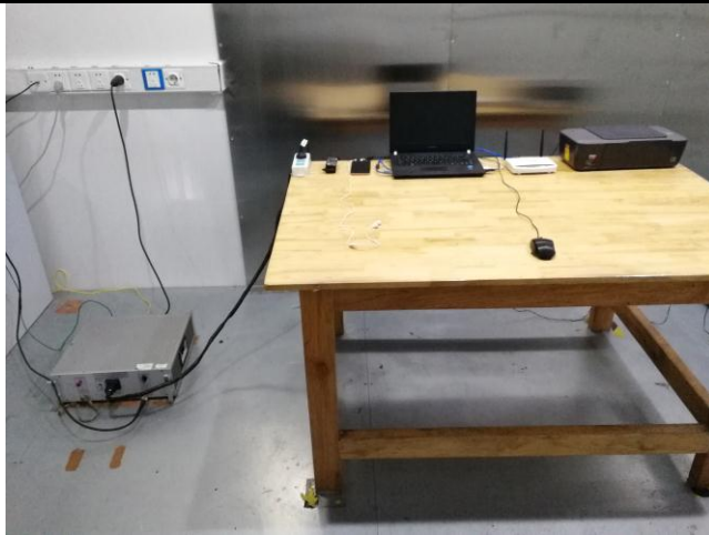
Conducted Emissions Test Setup – Front View
