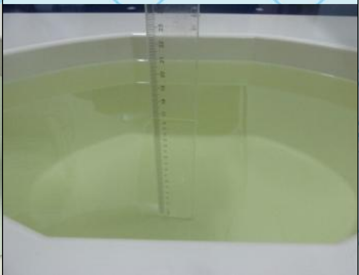
Photo 14: 1800~1900MHz Liquid Depth \geq 15.0\text{cm}
