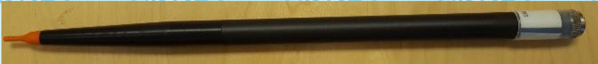
Figure 2 – MVG COMOSAR Dosimetric E field Dipole
