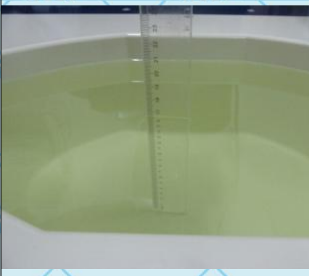
Photo 15: 2450MHz Liquid Depth \geq 15.0\text{cm}
