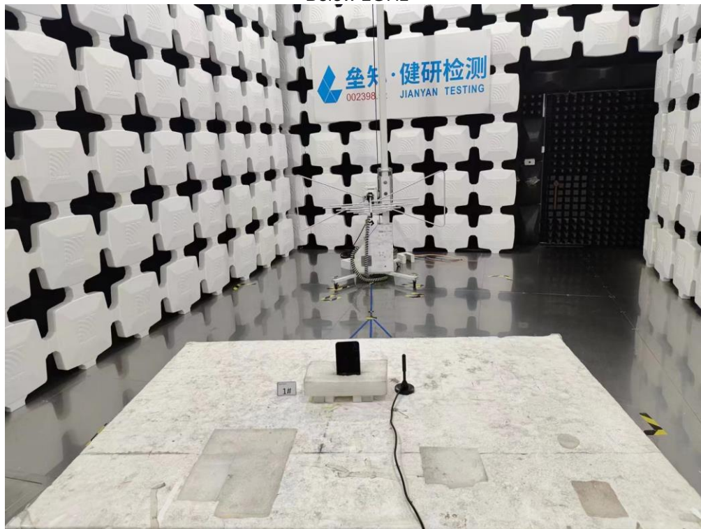
Radiated Spurious Emission Below 1GHz
