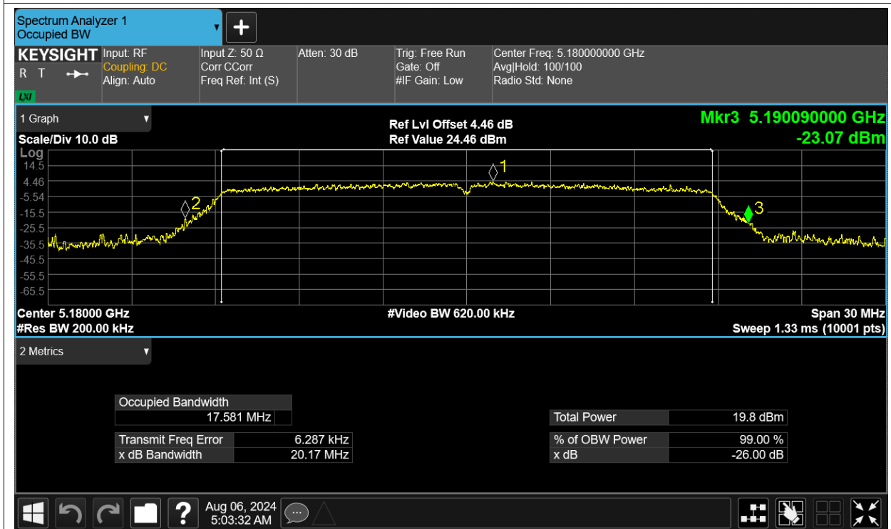
-26dB Bandwidth NVNT n20 5200MHz Ant1
