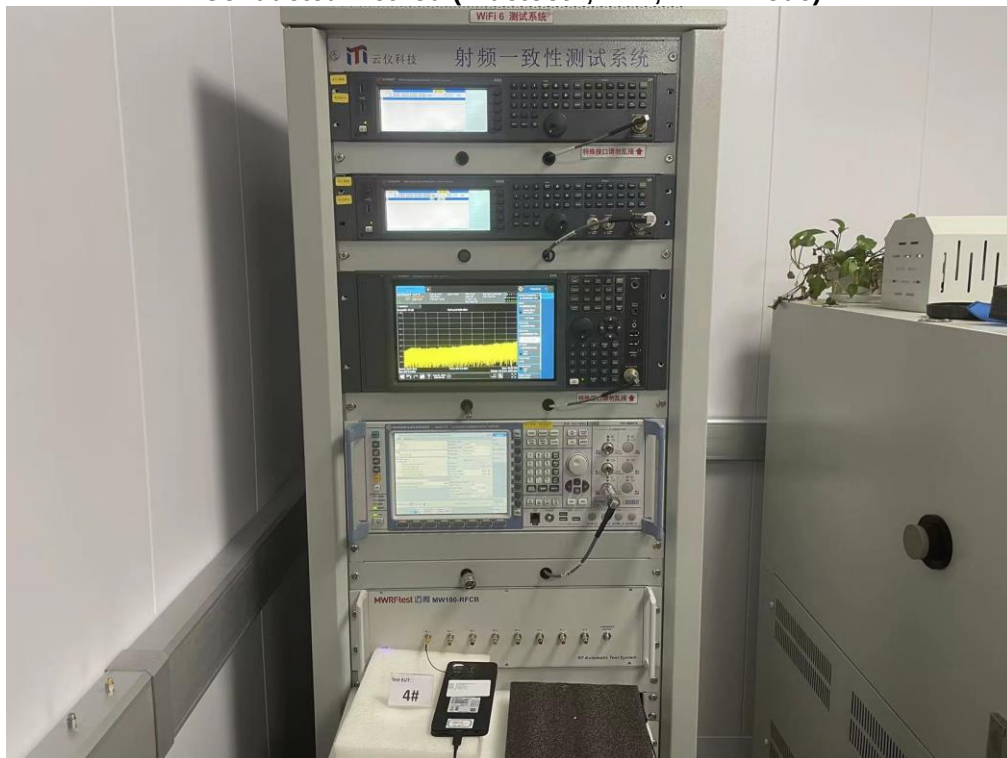
Conducted method (Bluetooth, BLE, Wi-Fi mode)
