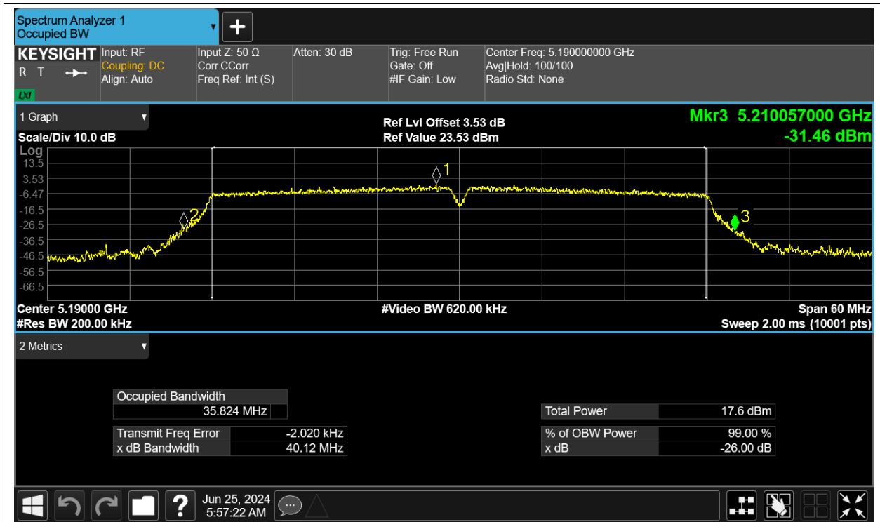
-26dB Bandwidth NVNT ac40 5230MHz Ant2
