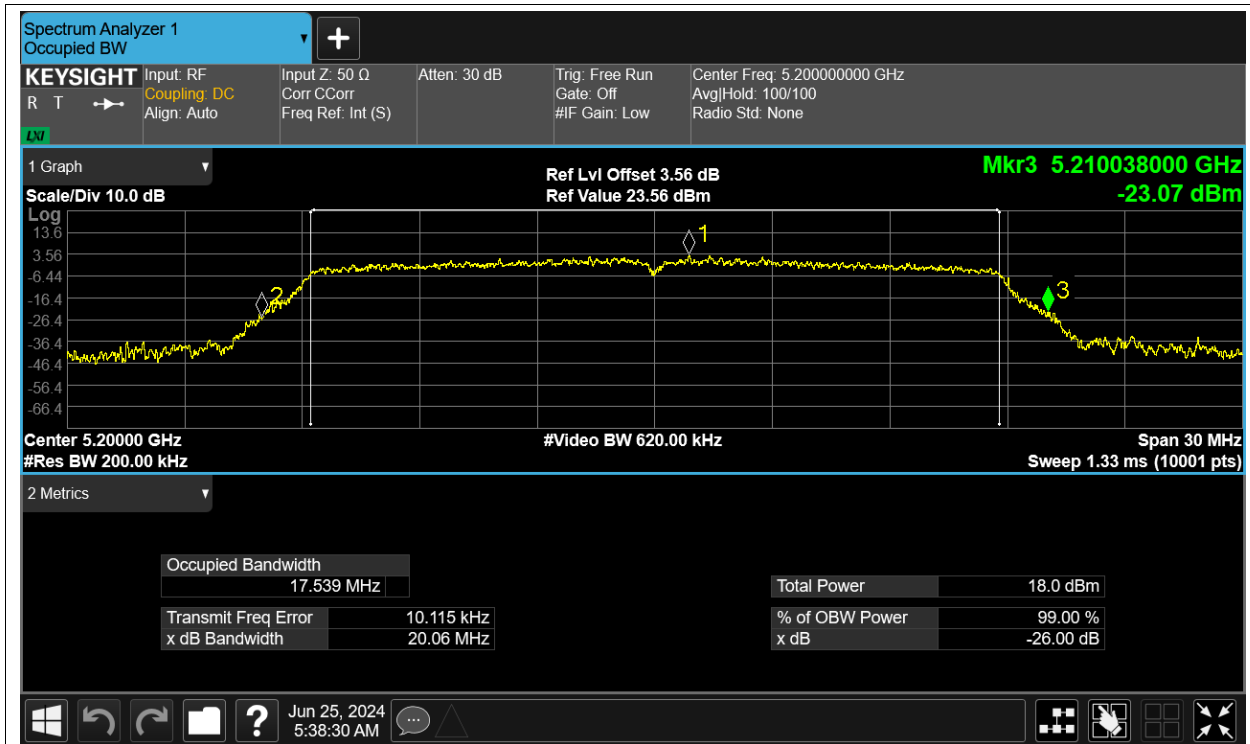
-26dB Bandwidth NVNT n20 5240MHz Ant2
