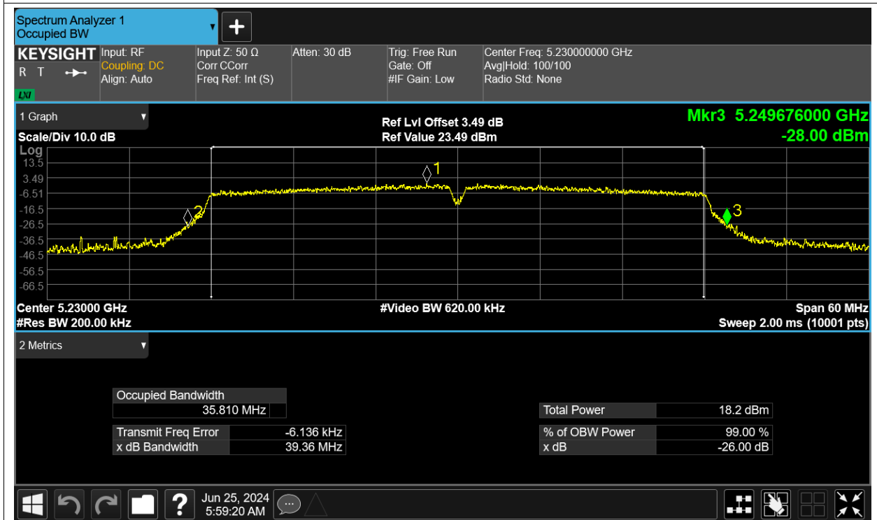
-26dB Bandwidth NVNT ac80 5210MHz Ant2
