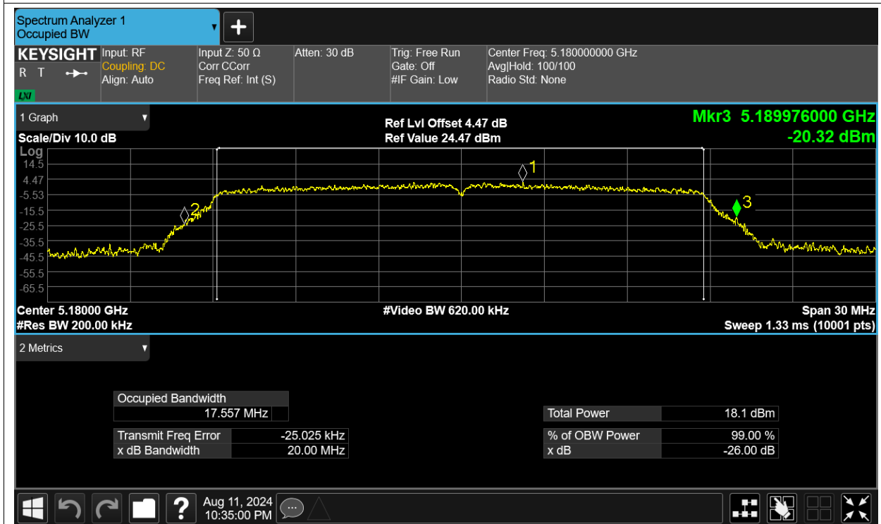
-26dB Bandwidth NVNT n20 5200MHz Ant1
