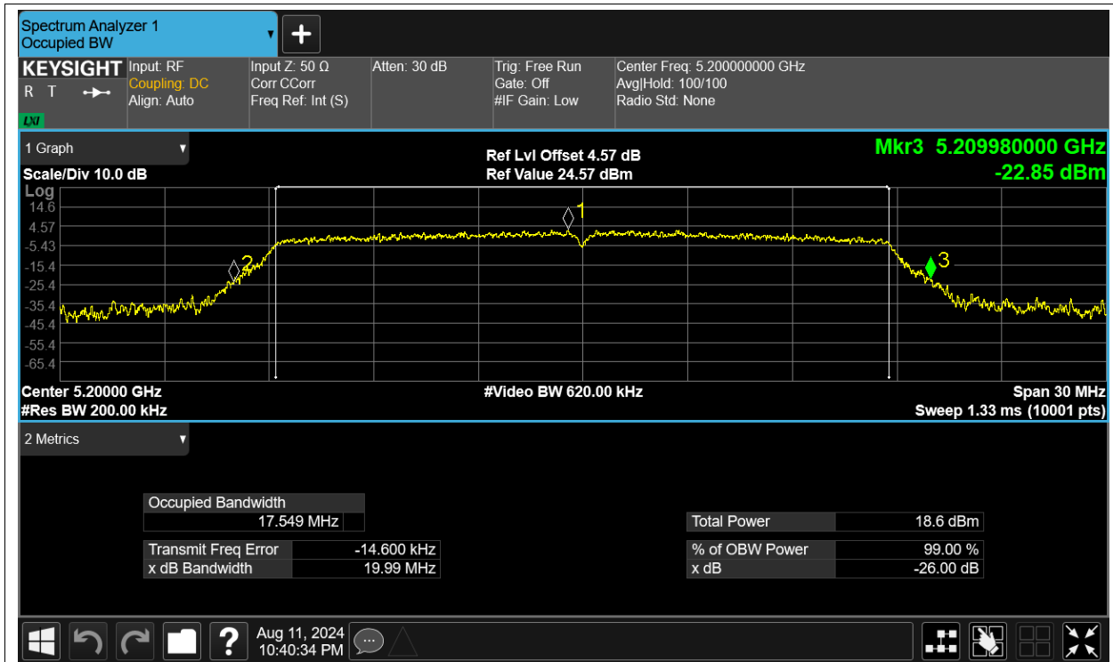
-26dB Bandwidth NVNT n20 5240MHz Ant1
