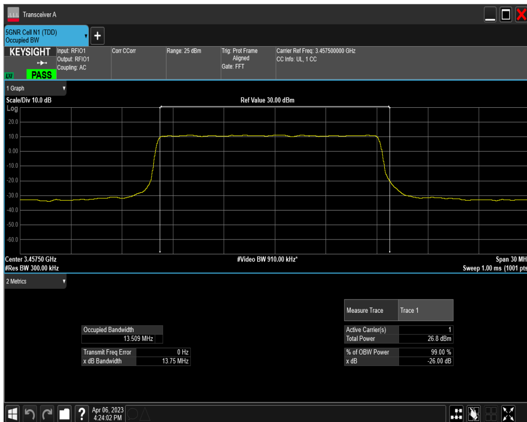
n77(3450-3550) SCS=30kHz DFT_QAM16 BW=15MHz Channel=630500 RB=36@0
