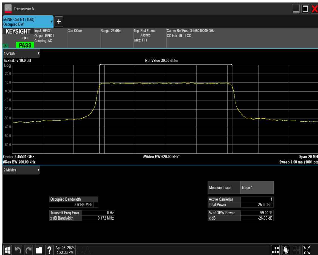
n77(3450-3550) SCS=30kHz DFT_QAM256 BW=10MHz Channel=630334 RB=24@0
