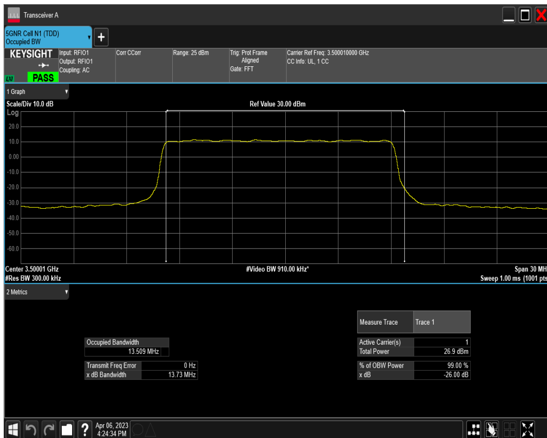
n77(3450-3550) SCS=30kHz DFT_QAM16 BW=15MHz Channel=633334 RB=36@0
