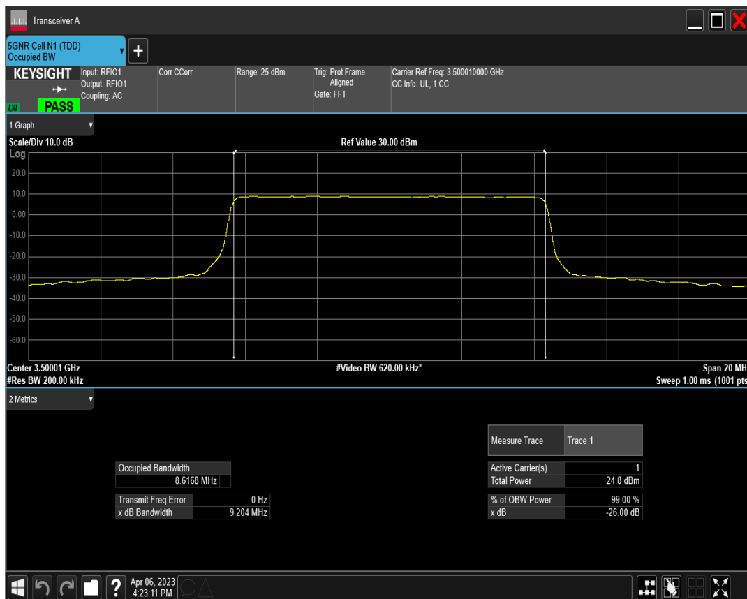
n77(3450-3550) SCS=30kHz DFT_BPSK BW=10MHz Channel=636332 RB=24@0
