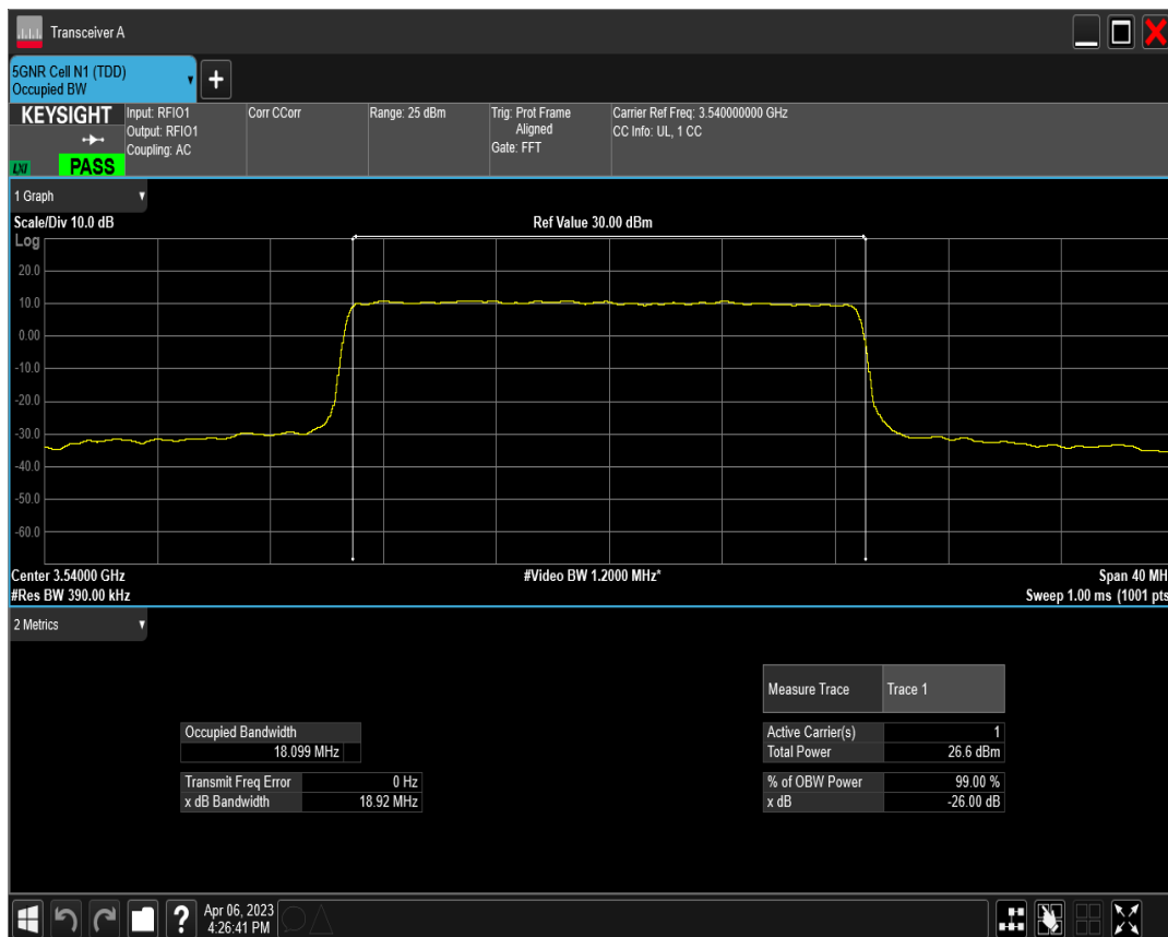
n77(3450-3550) SCS=30kHz DFT_QAM16 BW=20MHz Channel=636000 RB=50@0
