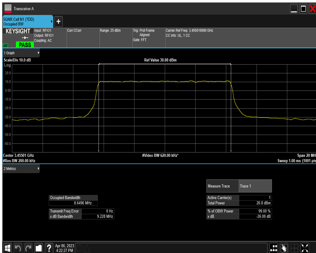
n77(3450-3550) SCS=30kHz DFT_QAM16 BW=10MHz Channel=630334 RB=24@0
