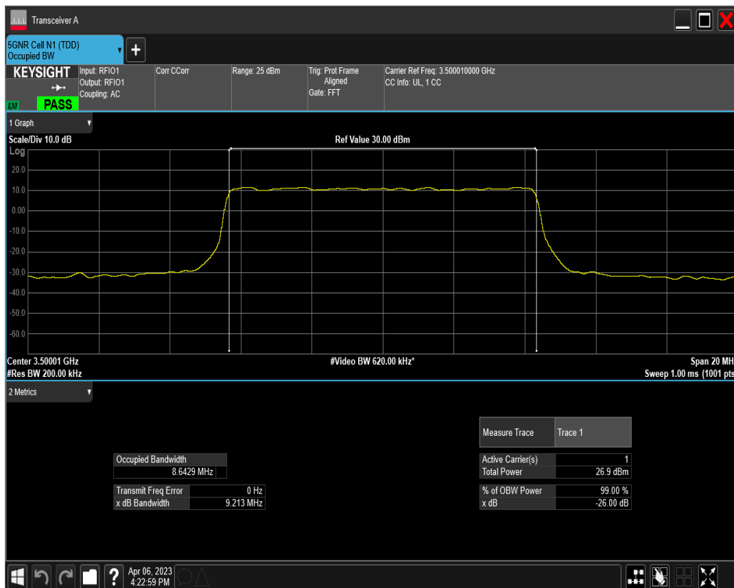
n77(3450-3550) SCS=30kHz DFT_QAM16 BW=10MHz Channel=633334 RB=24@0
