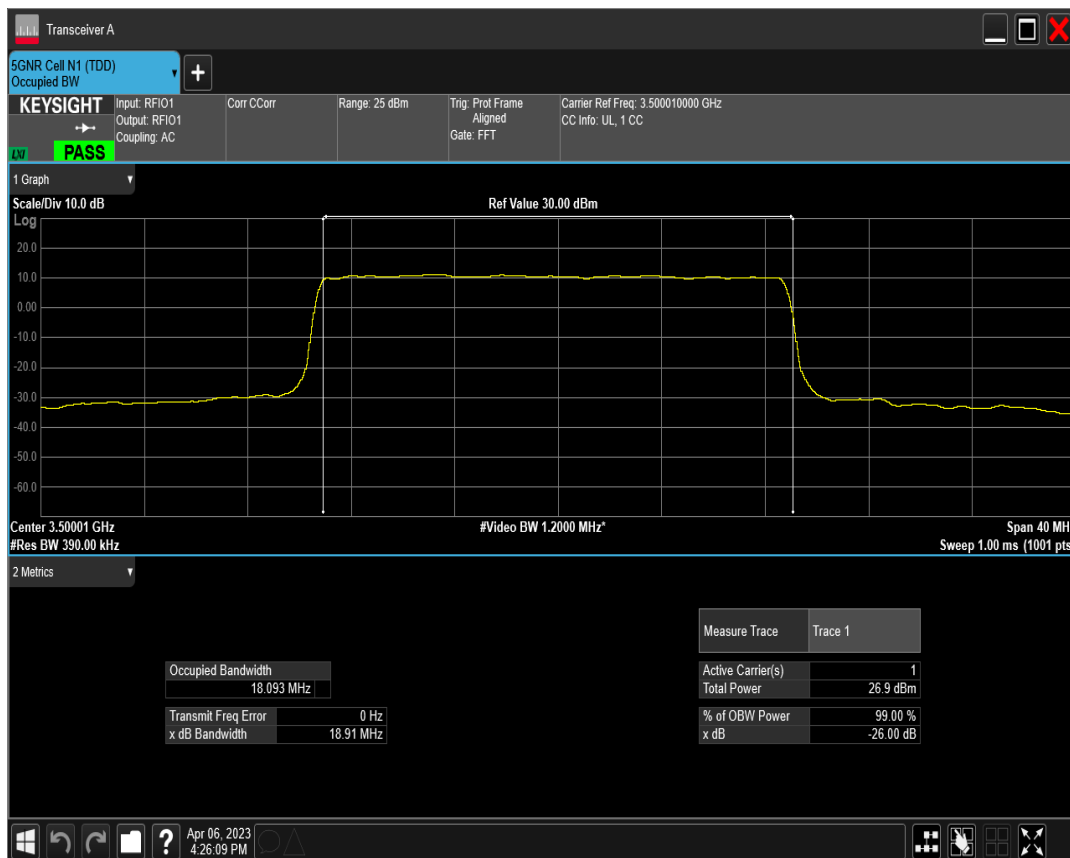
n77(3450-3550) SCS=30kHz DFT_QAM16 BW=20MHz Channel=633334 RB=50@0
