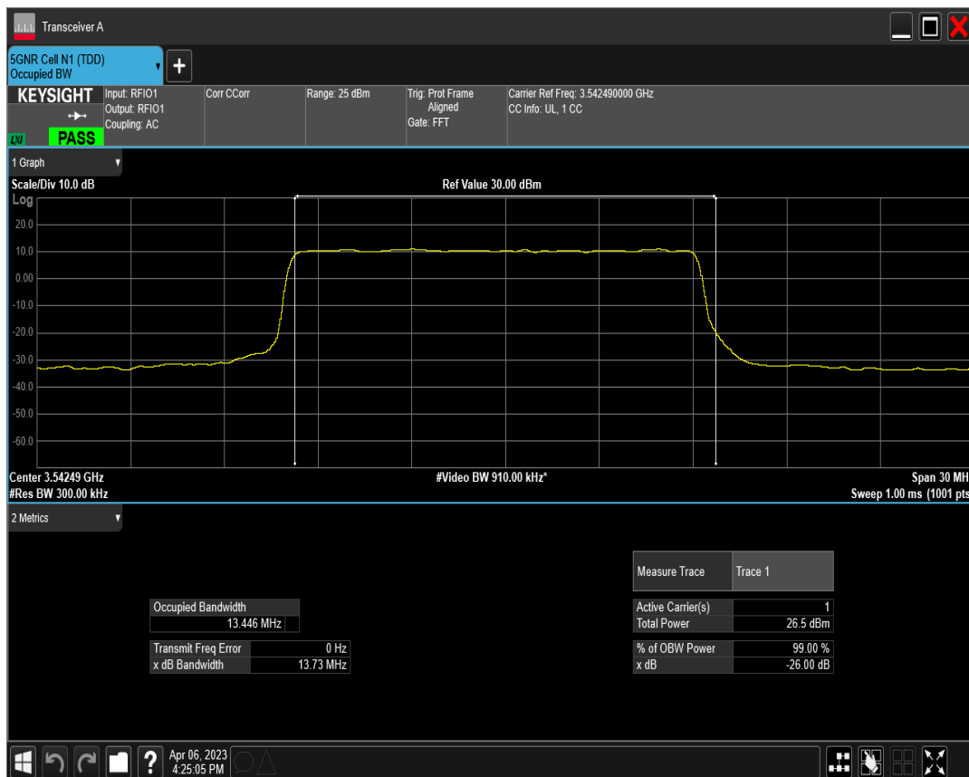
n77(3450-3550) SCS=30kHz DFT_QAM16 BW=15MHz Channel=636166 RB=36@0
