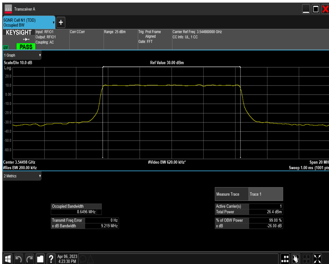
n77(3450-3550) SCS=30kHz DFT_QAM16 BW=10MHz Channel=636332 RB=24@0
