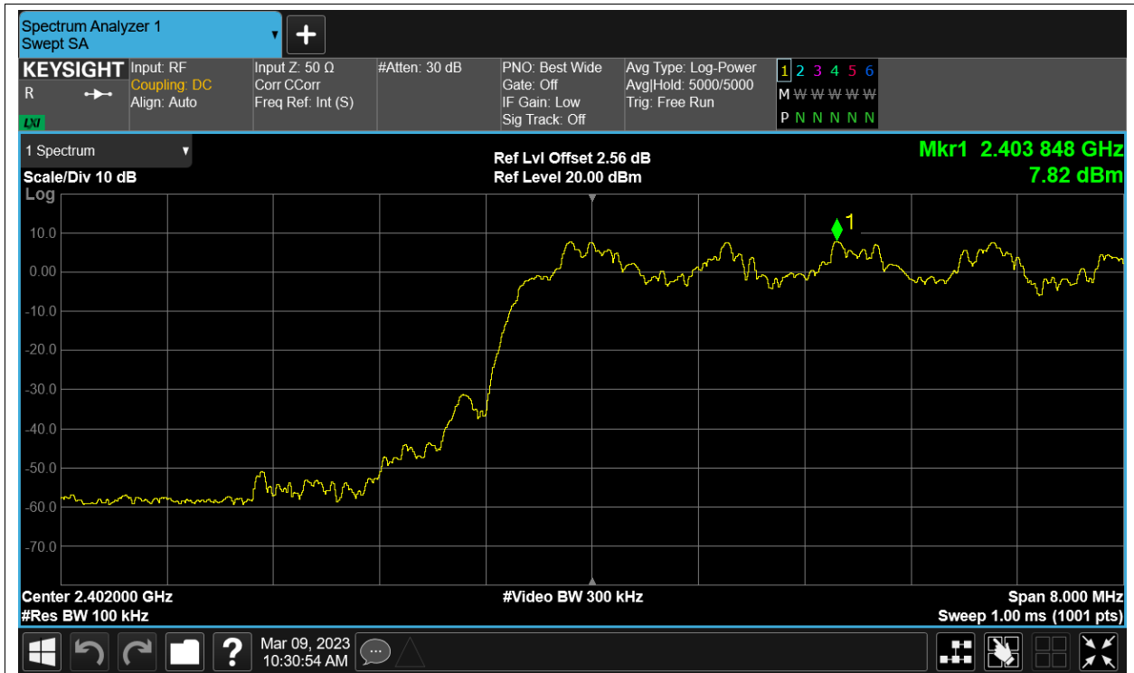
Band Edge(Hopping) NVNT 3-DH1 2402MHz Ant7 Hopping Emission
