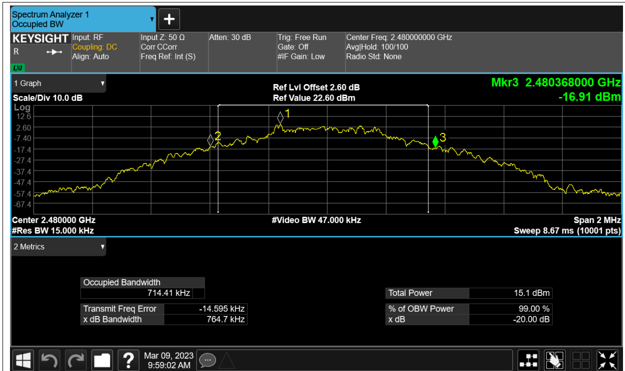
-20dB Bandwidth NVNT 2-DH1 2402MHz Ant7
