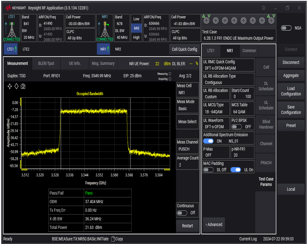
n78 SCS=30kHz DFT_QAM64 BW=50MHz Channel=636666 RB=128@0
