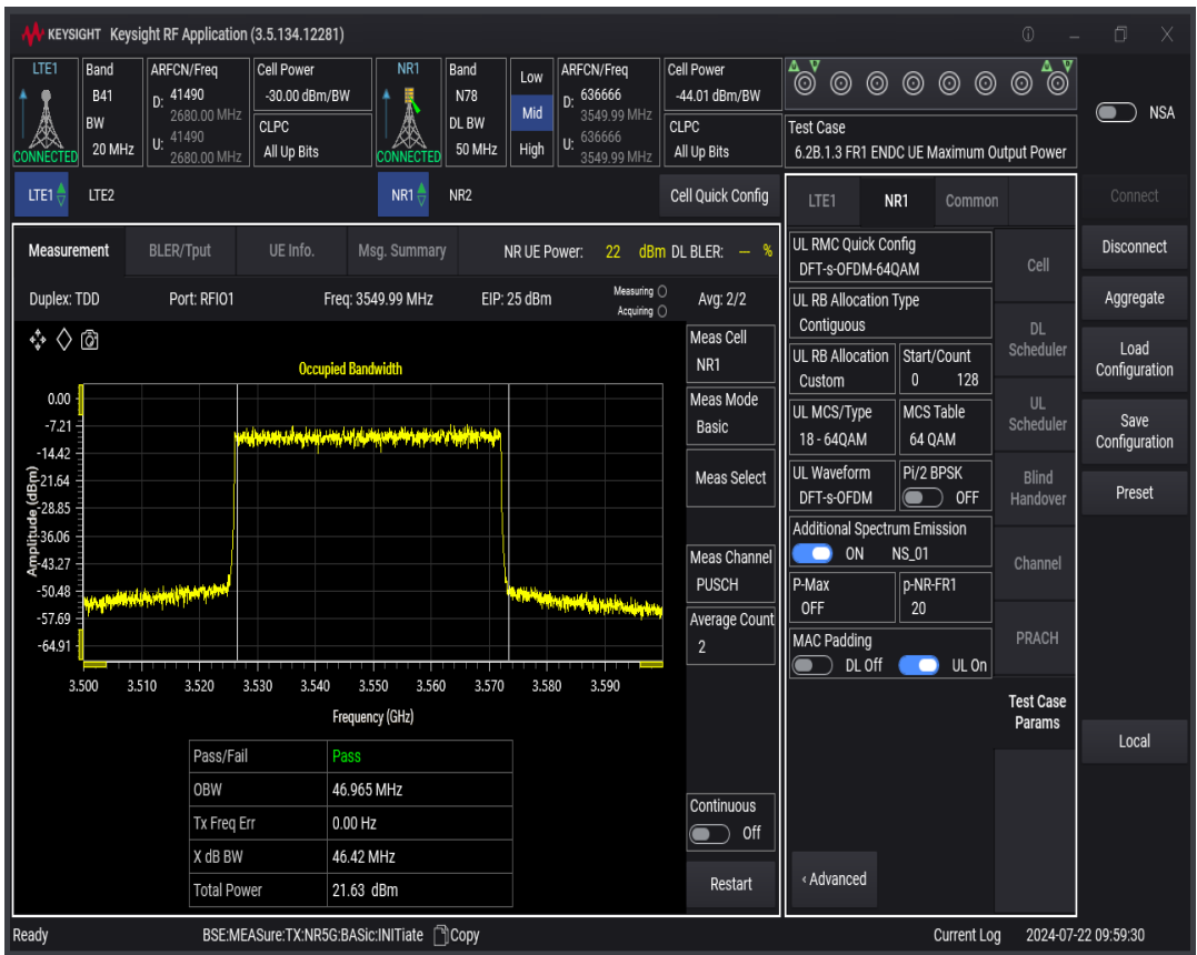
n78 SCS=30kHz DFT_QAM64 BW=60MHz Channel=636666 RB=162@0
