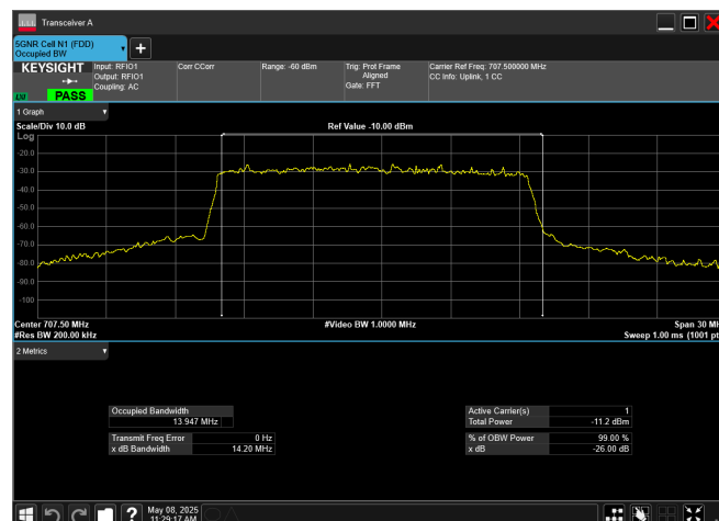
n12_15MHz_15kHz_707.5MHz_DFT-s-OFDM 64 QAM_RB75@0
