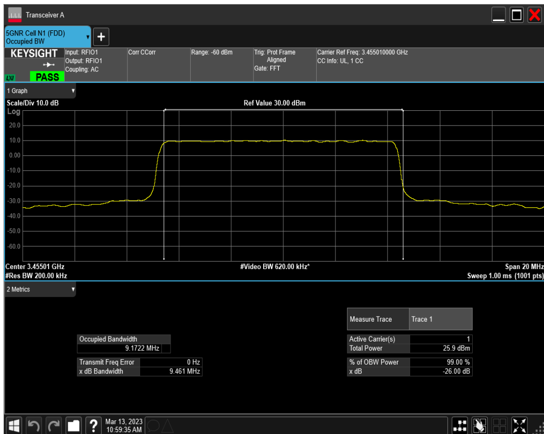
n77(3450-3550) SCS=15kHz DFT_QAM16 BW=10MHz Channel=630334 RB=50@0
