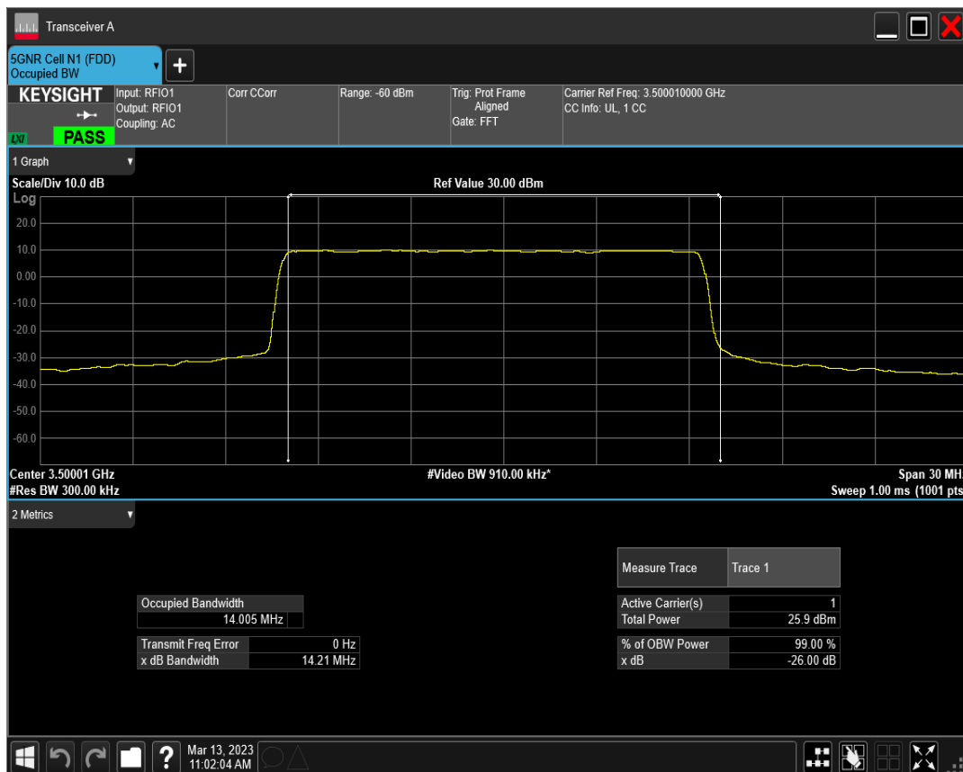
n77(3450-3550) SCS=15kHz DFT_QAM16 BW=15MHz Channel=633334 RB=75@0
