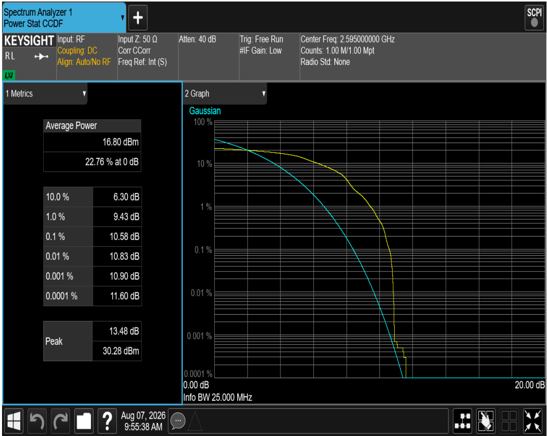
Band41(2535-2655) QAM16 BW=5MHz Channel=40640 RB Size=1 Position=#0
