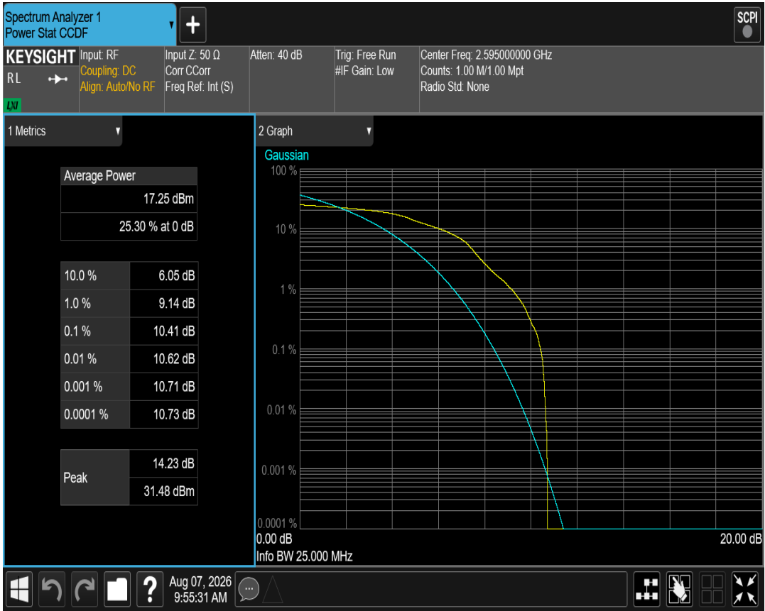
Band41(2535-2655) QAM16 BW=20MHz Channel=40640 RB Size=1 Position=#0
