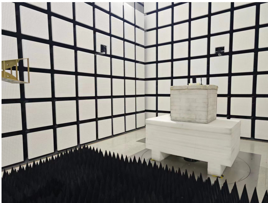
Radiated Emission Above 1GHz View
